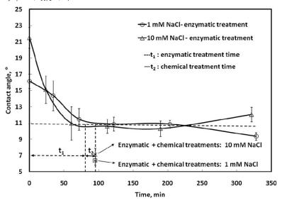
**Figure 3.**Effect of enzymatic treatment on the contact angle of the cellulose coated-gold sensor surfaces with the time.
