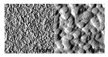
**Figure 1.** Atomic force microscopy images of the cellulose film with a scan size of  $5 \times 5 \,\mu m$  (left) and  $1 \times 1 \,\mu m$  (right).
