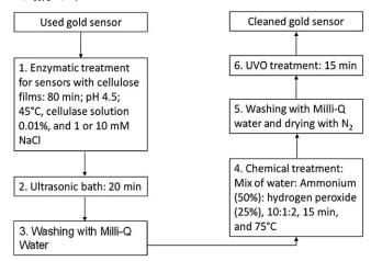
**Figure 2.**Block diagram of the proposed protocol of combined enzymatic and oxidative treatment for sensor cleaning and reuse.
